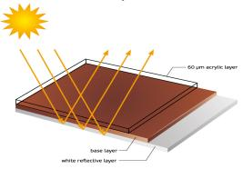
This is also one of the decisive features of the laminate and why it outperforms paint, because due to its multifunctional layers it achieves the highest Heat Build Up reduction and offers thanks to the different embossing's also a very high scratch resistance.
