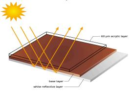
This is also one of the decisive features of the laminate and why it outperforms capstock, because due to its multifunctional layers it achieves the highest Heat Build Up reduction and offers thanks to the different embossing's also a very high scratch resistance.
